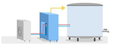
**Figure A.6** – Sample cold storage technology, where cold store (middle) was cooled via compressor (left) when electricity was available (in parallel to cooling the tank) and directly cools tank (right) during an outage without requiring electricity.
