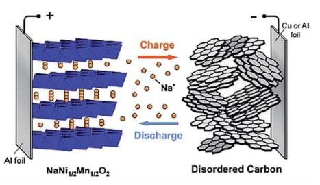
FigureA.4 - Schematic of sodium ion batteries with a layered transition metal oxide cathode and carbonaceous anode [28]
