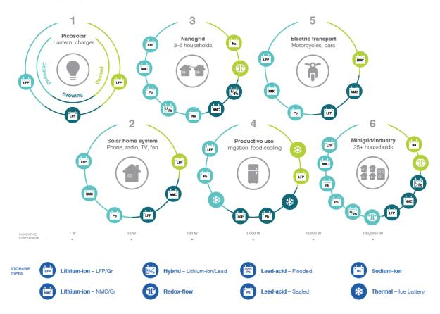
**Picosolar** – Small portable devices with low energy and power requirements tolerate high capacity cost lithium-ion for longer cycle life
