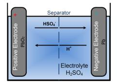
Figure A.1 - Principle of the discharge and charge process in a Lead-acid cell [25]
